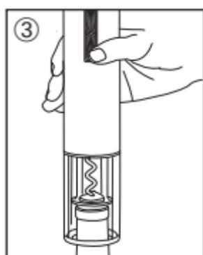
③ Keep the lower part of the start button pressed and apply a little downward pressure at the same time. The spiral turns into the cork and pulls it out. Once the cork is completely pulled out of the bottle, the corkscrew stops automatically. Release the start button and remove the corkscrew from the bottle.
