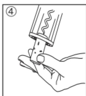
④ To twist the cork out of the corkscrew, keep the upper part of the start button pressed.
